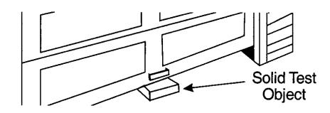
When the door reverses, remove the test object and run the full cycle of open and close of the door. Door should not reverse when it comes to the fully closed position.
